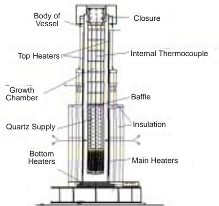
After sealing the vessel, the autoclave is heated to operating conditions with the use of external, resistance heaters. Typical operating conditions are between 300 and 400°C. The internal pressure developed is controlled by the temperature and the amount of solution added to the autoclave.
