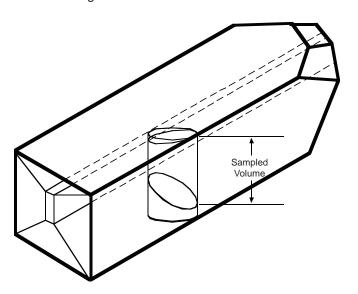
with six 6.35mm diameter circles, each bar is placed on a black background with the minus-X surface facing up. Using side illumination and index matching oil if necessary, each of the marked sites are examined under a stereoscopic microscope with calibrated reticle scales. The focal plane of the microscope is adjusted through the x-height of the bar such that the sampled volume is as indicated in the figure.
